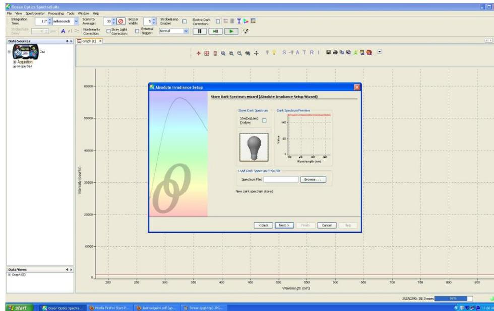
10. Completely block the light source for a dark spectrum. Click
