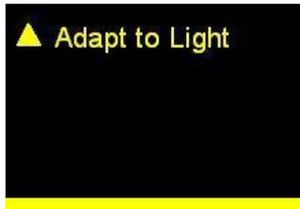
2. Point the probe at your sample (LED or other emissive light source) and press the ▲ key for the Adapt to Light selection. This starts the optimization procedure to adjust the Jaz instrument for the appropriate lighting conditions. Once Jaz has finished (within a few seconds), the following screen appears:
