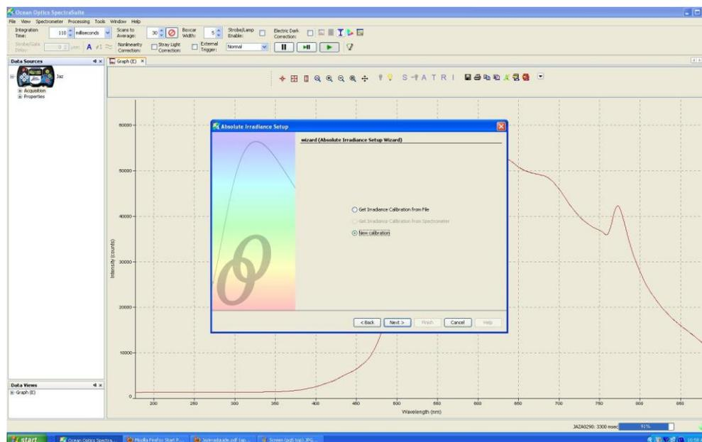
7. Select **New calibration** since you are calibrating the spectrometer with a light source. Click **Next**.
