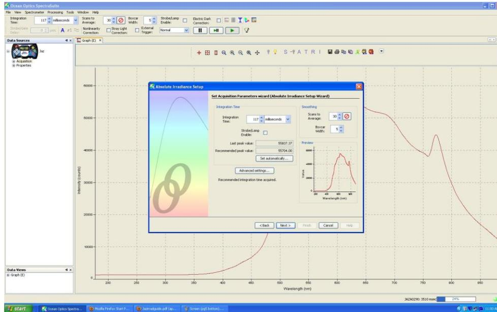
8. Set the spectrometer for the optimal signal-to-noise ratio by clicking **Set Automatically** or making the following individual selections:
