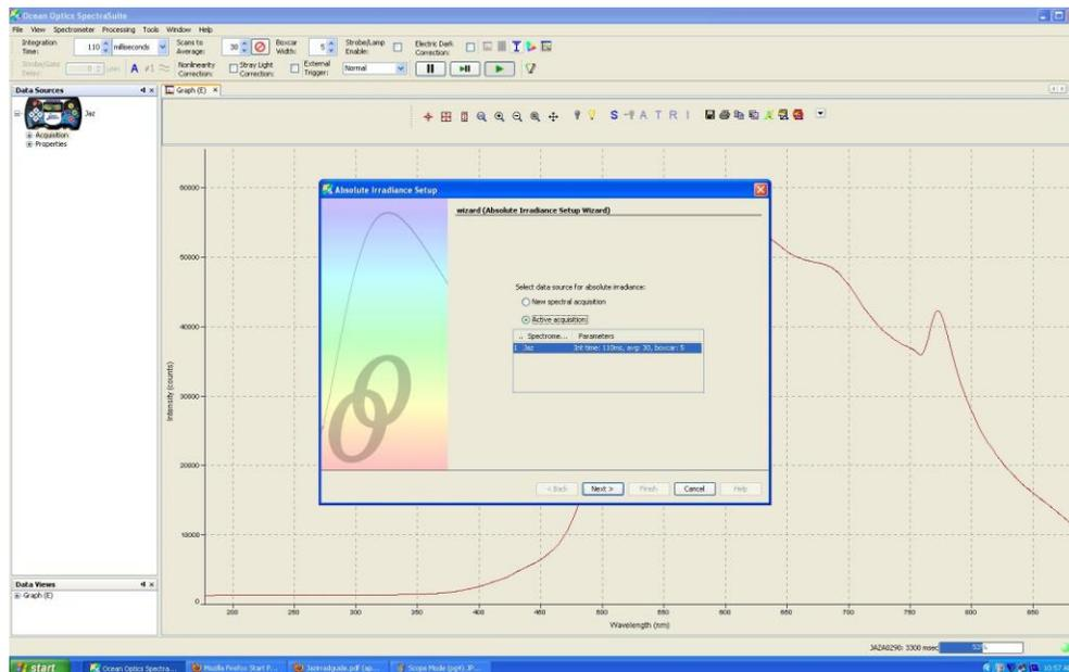
6. Select the desired spectrometer to set up the measurement. Click **Next**.
