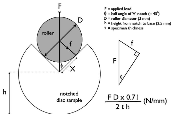
Fig. 1 – Schematic representation of how the torque to initiate failure (*T*) is derived. The specimen has a 90° V notch,  $\phi = 45^\circ$  and  $\sin 45^\circ = 0.71$ .
