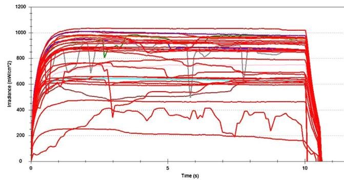
**Fig. 2 – Results – irradiance delivered by 10 operators (5 staff and 5 students; 3 tests per operator) to the occlusal cavity floor of tooth 27 in a MARC-PS® unit (Bluelight Analytics Inc., Halifax, NS) using the Bluephase® light for 10 s at high power setting. The distance between the cusp tips and the sensor in the cavity floor of tooth 27 was 4 mm. Inter-incisal opening of the mannequin head was fixed at 43 mm.**
