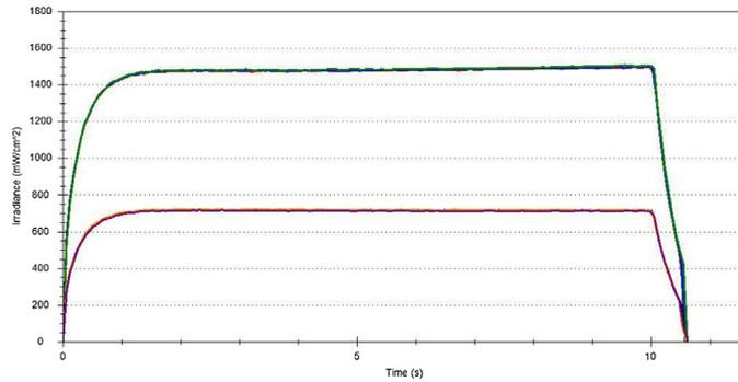
**Fig. 4 – Results – irradiance delivered (n = 3 tests at each distance) by the Bluephase® light at used for 10 s at high power setting at 0 mm and 7 mm distances from the light sensor (4 mm diameter) of a MARC-RC® unit (Bluelight Analytics Inc., Halifax, NS).**
