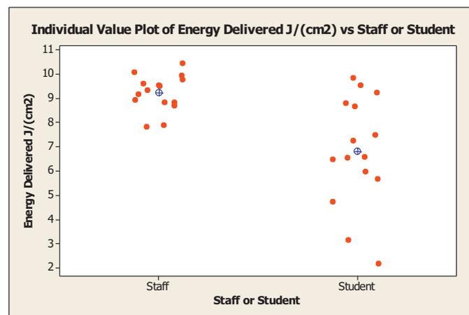
**Fig. 3 – Results – plot of the individual radiant exposure (J/cm<sup>2</sup>) results for the ten operators. Circled crosshairs show the mean for each of the 2 operator groups. Note the higher scatter and lower mean energy delivered by the less experienced student operators.**
