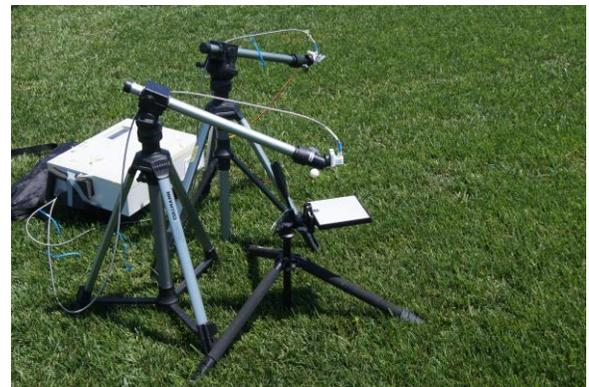
Prototype of the autonomous fluorescence measurement system during a test run over pasture in Italy.
