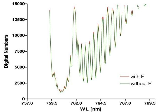
O<sub>2</sub>A Fraunhofer line at 760 nm, measured with an Ocean Optics QE spectrometer. The red line shows the signal with and the green without fluorescence.
