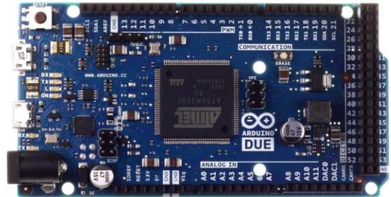
Arduino DUE open source micro-controller, operating spectrometer, cooling system and environmental sensors
