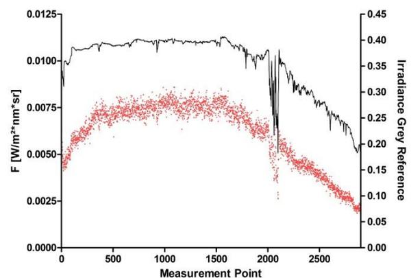
Looking into plants in a novel way - On the right, a preliminary daycourse of F (red dots) measured by the prototype is shown for vegetation. The black line represents the sun irradiance. Note how F drops with an incoming cloud.
