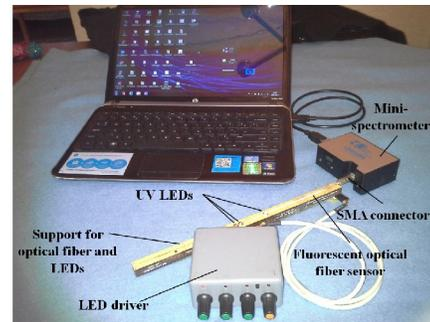
**Figure 2b.** Actual picture of the whole system illustrated in Fig. 2a.
