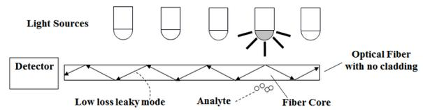
**Figure 1b.** Light source probing a bare core optical fiber. The analyte, e.g., nitrate in water, is behind the optical fiber.
