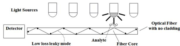
**Figure 1a.** Light source probing a bare core optical fiber. The analyte, e.g., nitrate in water, is between the source and the optical fiber.
