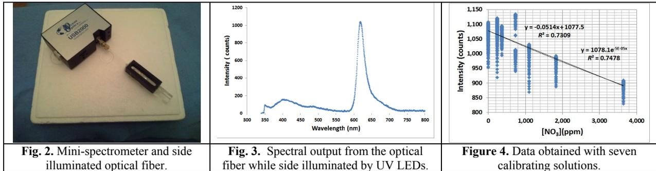
Seven nitrate solutions were prepared to calibrate sensor with the following concentrations: 0, 233, 365, 729, 1,101, 1,823, 3,645, 5,504, 7,290 and 9,149 ppm. As each solution was poured into the black container, a light intensity measurement was taken nearby the peak wavelength: at the 600 nm reading which corresponds to a 300 nm wavelength (see Fig. 4).
