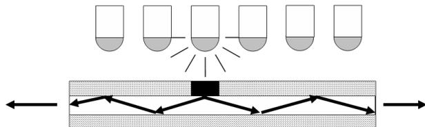
**Figure 1a.** Light source #3 probing a fluorescent cladding optical fiber and its associated fiber section.
