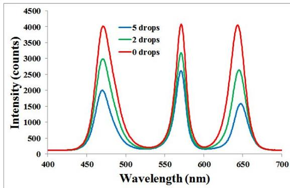
Fig. 3a. Spectral curves of the first, second and third sensing points of the fluorescent cladded optical fiber.
