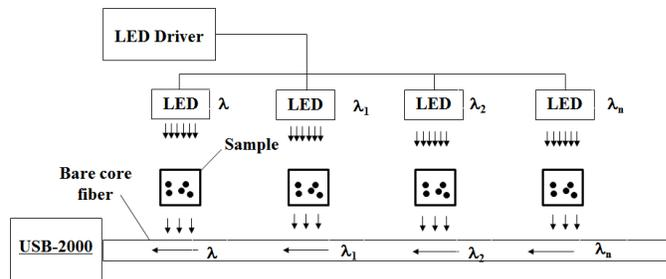
**Figure 2a.** Simultaneous multiple point sensing with a bare core optical fiber (not in scale).
