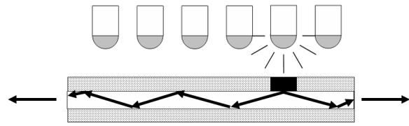
**Figure 1b.** Light source #5 probing a fluorescent cladding optical fiber and its associated fiber section.
