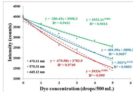
Fig. 3b. Spectral curves of the first, second and third sensing points of the fluorescent cladded optical fiber.
