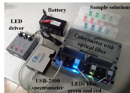
**Figure 2b.** Actual picture of the whole system illustrated in Fig. 2a.
