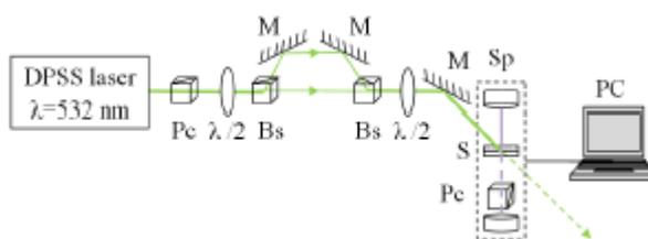
**Fig. 1.** Experimental setup for studying the absorption spectrum while irradiating the sample with polarized and non-polarized 532 nm laser light: Bs – beam splitter, F – neutral density filter, L – lens,  $\lambda/2$  – half wave plate, M – mirror, Pc – polarisation cube, PC – computer, S – sample, Sp – Ocean Optic HR4000CG spectrometer
