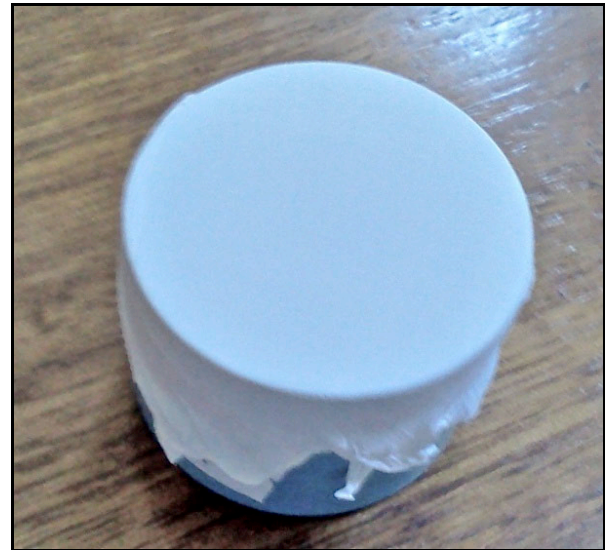
Fig. 12. Teflon's layers over the PVC cylinder.
