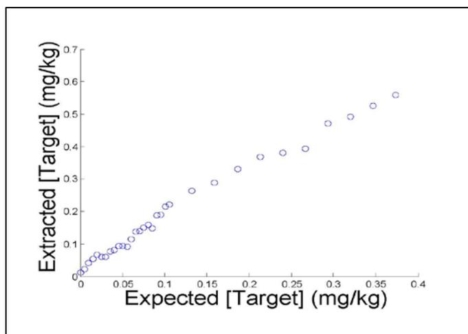
Figure 6: Extracted concentration for a target drug measured by the Zenascope is shown relative to expected absorption calculated from known concentrations.
