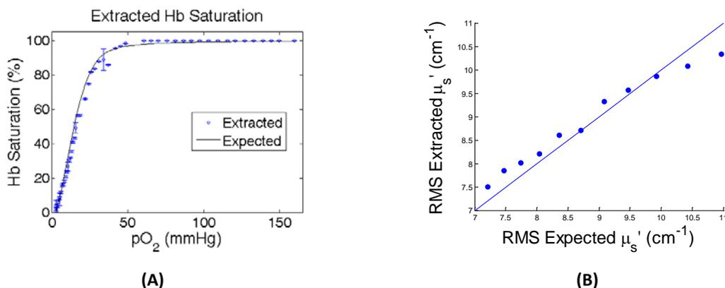
**Figure 4:** Expected and extracted results achieved with the Zenalux Algorithm in turbid suspensions containing varying concentrations of hemoglobin and polystyrene microspheres. (A) Zenascope measured hemoglobin saturation (%HbO<sub>2</sub>) is shown relative to expected values. (B) Zenascope measured scattering ( $\mu_s'$ ) is shown relative to expected scattering.
