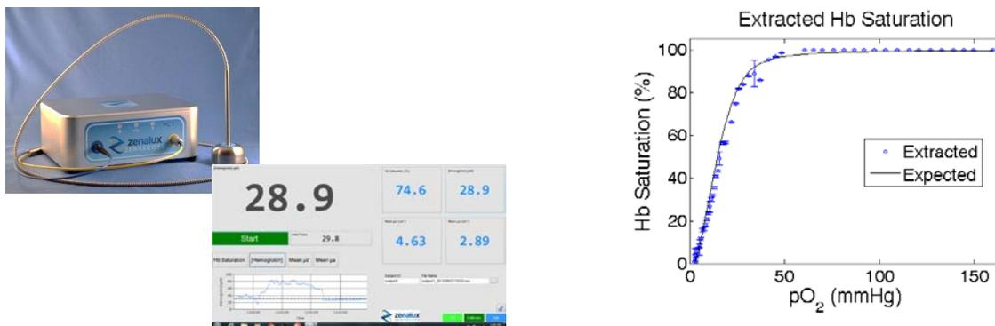
Figure 1. The Zenascope system, software output and an example measurement in which extracted hemoglobin saturation (the percentage of oxygenated hemoglobin to total hemoglobin content) is shown relative to expected values.
