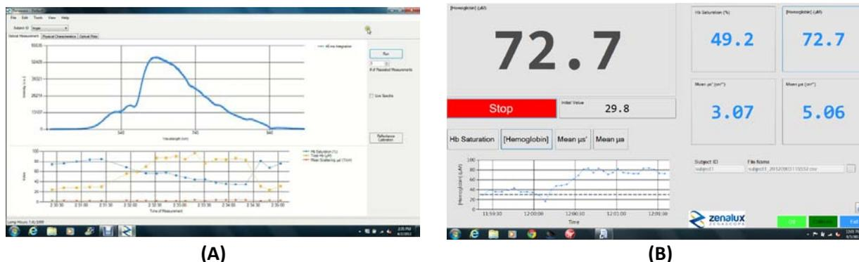
**Figure 5:** Zenascope converts classical optical reflectance spectra into quantitative measure of THb, Hb saturation, and scattering. Users can monitor and record the detailed tissue spectra and the outcomes associated with them (A); or simply monitor and record the outcomes with a more user friendly interface (B).
