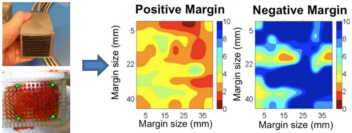
Figure 11. 49-channel probe and excised breast specimen in specimen holder (green dots indicating margin) and resulting parameter maps of beta carotene to scattering for a positive and negative margin[15].
