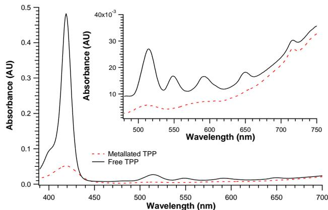
**Figure 4.** Typical UV-Vis absorption spectrum of a porphyrin (student data). The intense Soret band appears around 420 nm and the weaker Q-bands (inset) appear in the 500-700 nm range.
