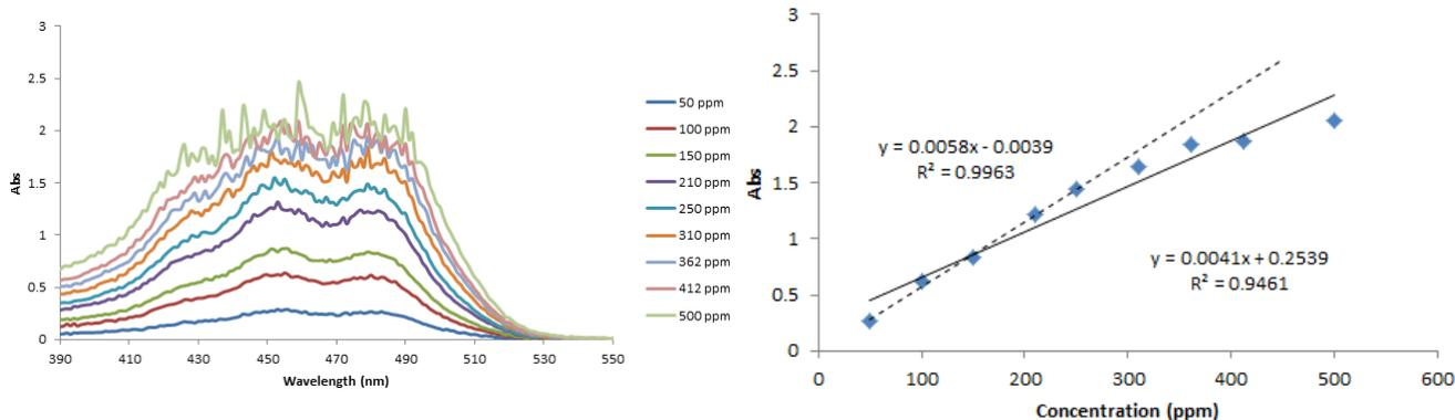
**Figure 7.** Left: Absorption spectra of fluorescein as a function of concentration from 390 to 550 nm recorded with the Ocean Optics USB650 Red Tide. Right: Beer's Law plot for fluorescein at 480 nm. The absorption of fluorescein increases linearly with concentration to approximately 1.5 O.D.
