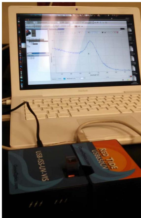
**Figure 8.** Experimental setup for the determination of the absorption spectrum of gold nanospheres.
