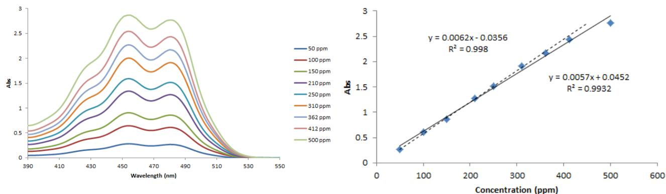
**Figure 6.** Left: Fluorescein absorption from 390 to 550 nm as a function of concentration recorded with the Cary 4000. Right: Beer's Law plot for fluorescein at 480 nm. The absorption of fluorescein increases linearly with concentration to greater than 2 O.D.
