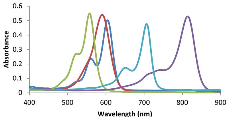
**Figure 3.** The absorption spectra of the cyanine dyes. Green: 1,1-diethyl-2,4-cyanine iodide, red: 1,1-diethyl-4,4-cyanine iodide, dark blue: 1,1-diethyl-2,2-carbocyanine iodide, light blue: 1,1-diethyl-4,4-carbocyanine iodide, purple: 1,1-diethyl-4,4-dicarbocyanine iodide.
