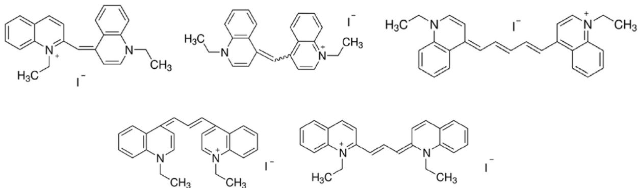
**Figure 1.** Structures of cyanine dyes. Clockwise from top left: 1,1'-diethyl-2,4'-cyanine iodide, 1,1'-diethyl-4,4'-cyanine iodide, 1,1'-diethyl-4,4'-dicarbocyanine iodide, 1,1'-diethyl-2,2'-carbocyanine iodide, 1,1'-diethyl-4,4'-carbocyanine iodide.
