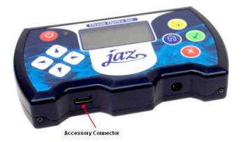
2. Connect the other end of the cable (with the DB15 connector) to the accessory being used.
