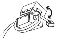
5. Snap the ferrite closed to lock it in place.
