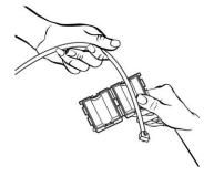
4. Loop the Ethernet cable through the ferrite twice.
