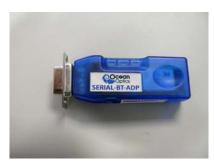
The adapters are used in pairs to replace a direct serial data cable connection anywhere in your laboratory or industrial system. Simply disconnect each end of the RS-232 cable and connect the correct adapters (male or female) to the equipment at each end of the link. See the example below using an STS spectrometer.
