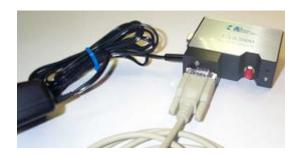
Figure 2: USB-CBL-PS 5-volt power supply and DB9 cable connected to USB2000 (shown) or HR2000 spectrometer using the USB-ADP-PC adapter
