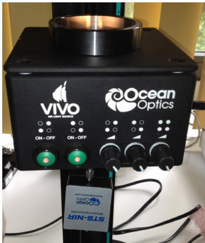
Figure 1: A high-power tungsten halogen source and a Shortwave NIR microspectrometer are mounted to an optical fixture to measure grain and other samples.
