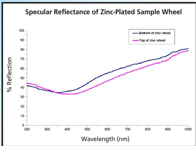
Figure 1: Zinc samples showed comparable reflectivity from both sides of the sample wheel.
