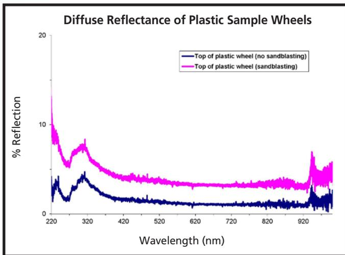
Figure 4: As expected, diffuse reflectance in both zinc and plastic wheels increased after sandblasting, presumably because the treated sample surfaces were rougher.
