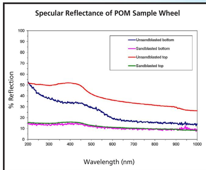
Figure 3: Sandblasting affected the reflectivity of plastic wheel samples, although not as dramatically as with the zinc wheels.
