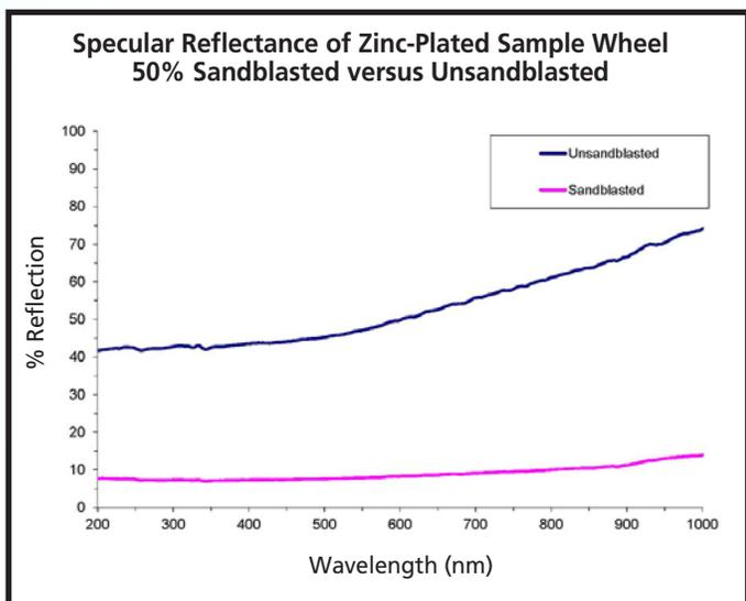
Figure 2: With all sample materials, sandblasting resulted in lower specular reflectance.
