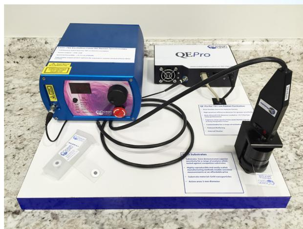
A modular SERS system like this can be configured for rapid, portable analysis of contaminants and is a convenient alternative to other screening techniques.
