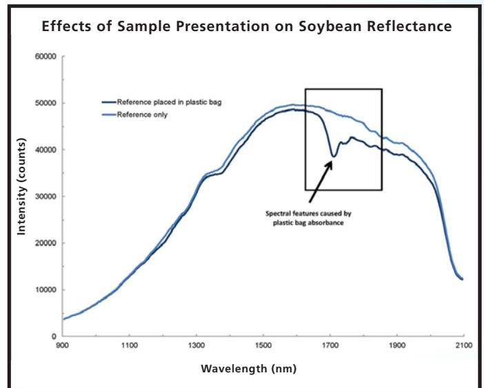
Figure 2: Accurate NIR measurements of food and other packaged samples require consideration of the effects of any packaging in the light path.
