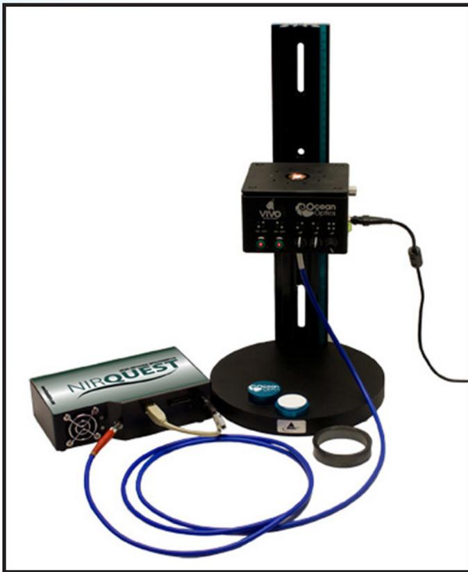
Figure 1: An NIR spectrometer is configured with light source and sampling fixture for diffuse reflection measurements.
