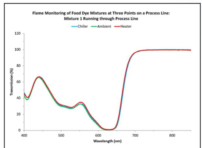
Figure 3: Spectra measured for the Mixture 1 solution were remarkably consistent across each temperature condition – chilled (24 °C), ambient (27 °C) and heated (30 °C).
