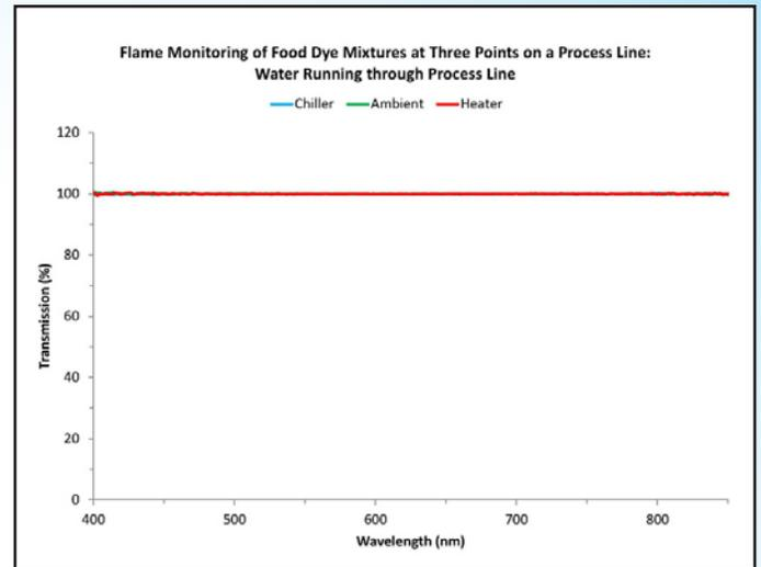
Figure 2: To establish a reference measurement for the experiment, water was measured in each of three temperature environments (chilled, ambient and heated).
