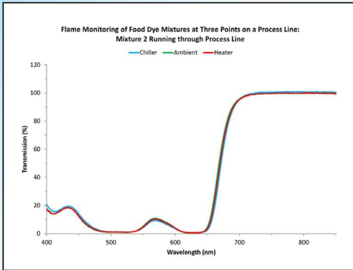
Figure 4: The Flame spectrometer produced consistent results across different temperature conditions, as these transmission spectra reveal.
