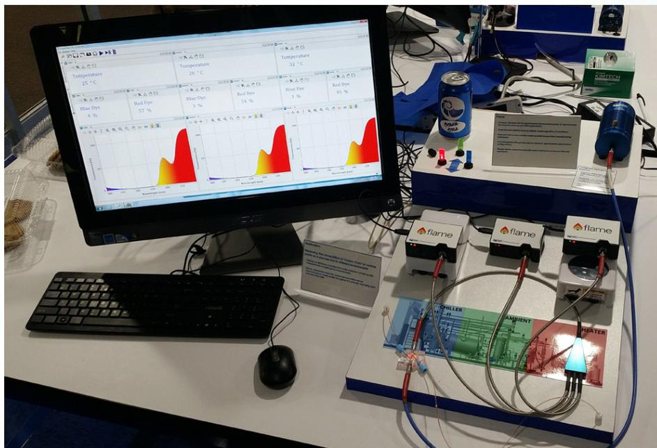
Figure 1: Several food dye mixtures were measured using Flame spectrometers in a simulated process line setup.
