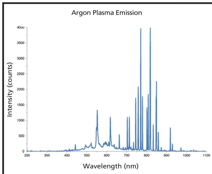
Figure 2: Emission of argon plasma is measured through a vacuum chamber window.
