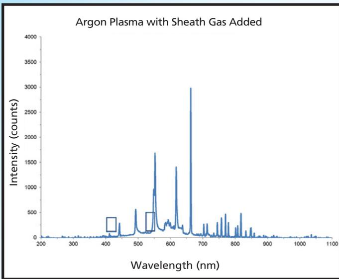
Figure 5: With the addition of sheath gas, argon emission characteristics are noticeably different below 400 nm and at ~520 nm.
