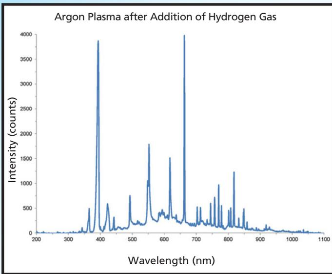
Figure 3: Adding hydrogen gas to the argon plasma changes its spectral properties.
