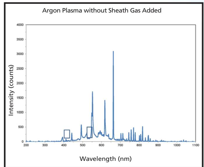
Figure 4: Argon plasma emission is measured in the vacuum chamber before the addition of sheath gas.
