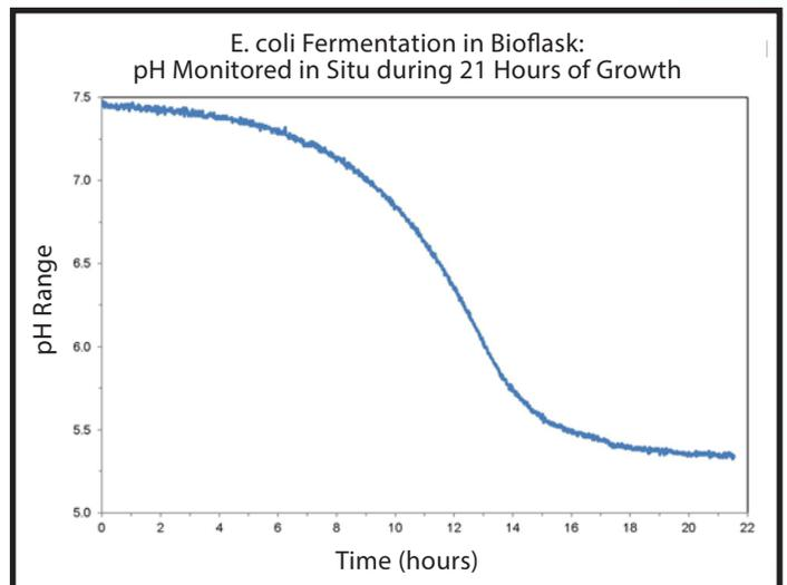
Figure 4: Over 21 hours of E. coli fermentation, pH levels drop as cell growth increases.
