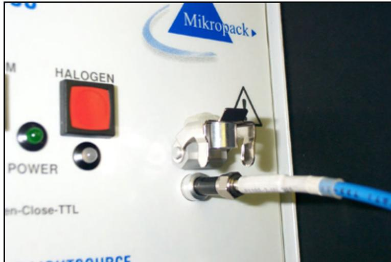
1. Locate the cap on the front of the DH-2000-CAL.
