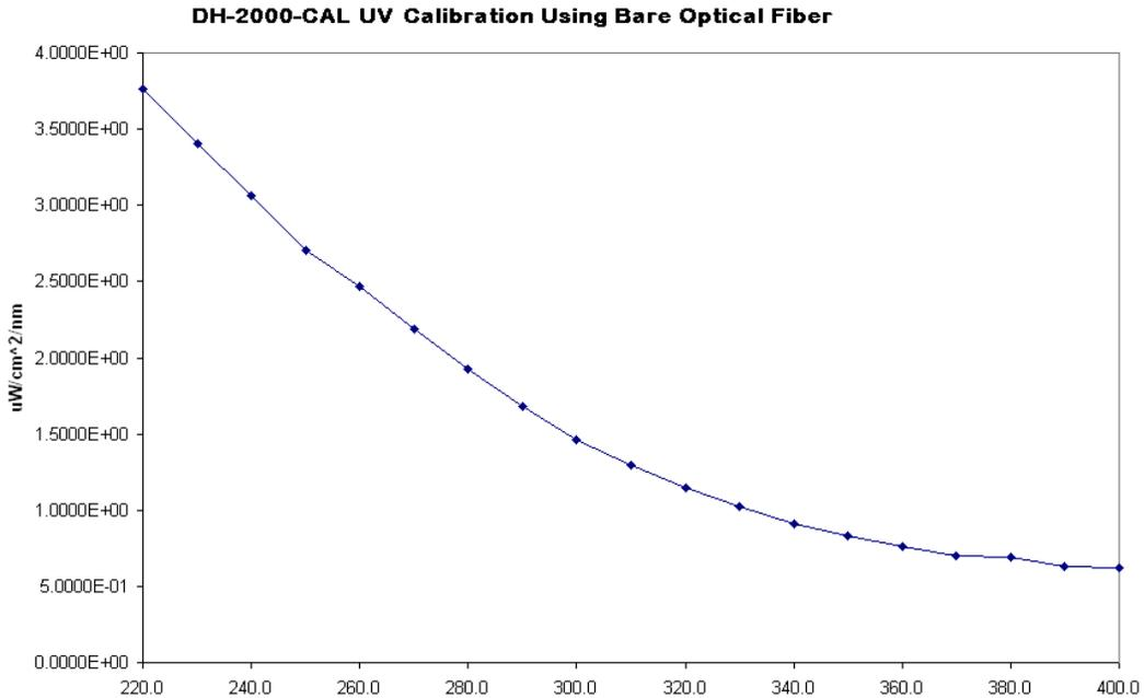
**Deuterium bulb spectral output using a bare SMA-terminated fiber**
