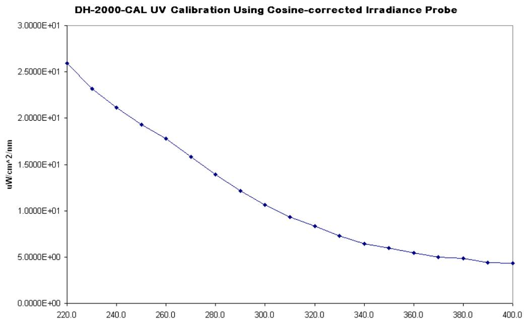
**Deuterium bulb spectral output using a CC-3 Cosine Corrector**
