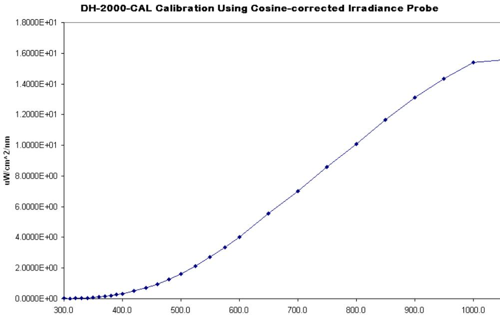
**Tungsten-Halogen bulb spectral output using a CC-3 Cosine Corrector**
