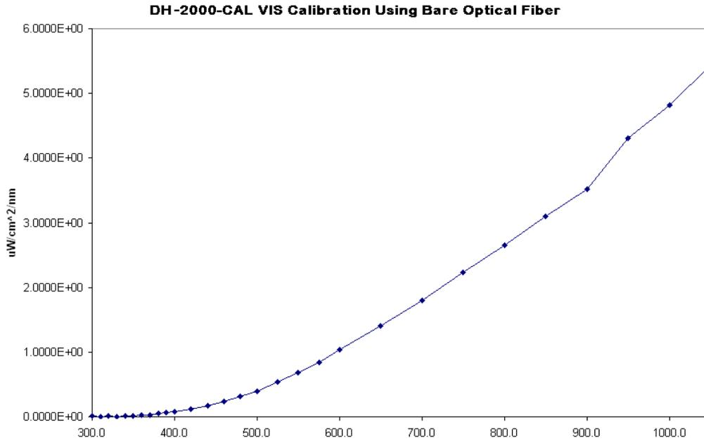
**Tungsten-Halogen bulb spectral output using a bare SMA-terminated fiber**
