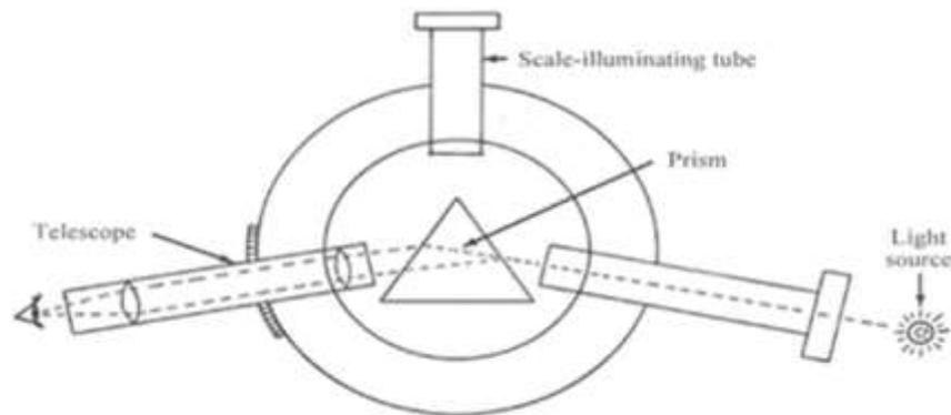
Figure 6: Diagram of a spectroscopy setup
