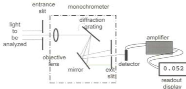
Figure 7: Diagram of a simple spectrometer
