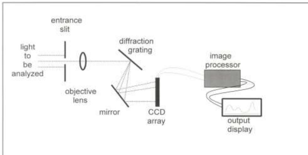
Figure 8: Diagram of a CCD Spectrometer
