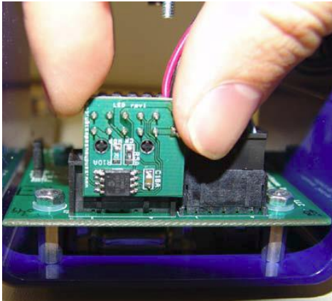
Removing the LED Connection Board
