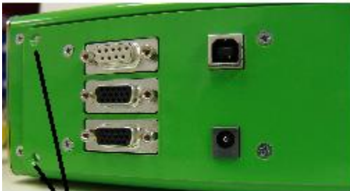
Screw holes to remove back panel
