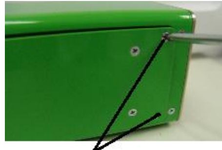
Screw holes to remove back panel
