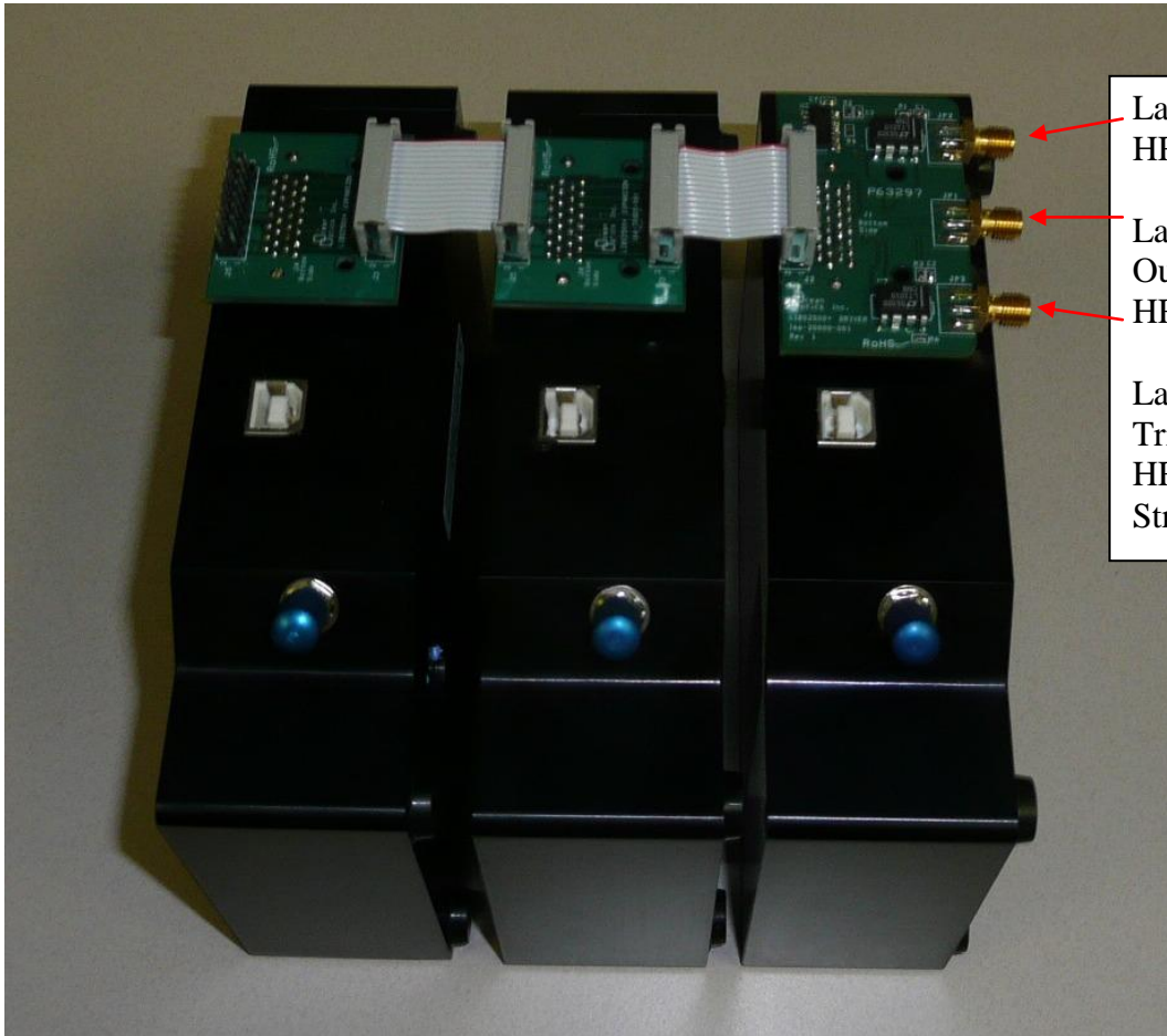
3-channel HR2000+ LIBS setup
