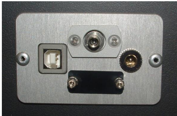
USB-connector to PC SMA-905 fiber connector DC-plug for spectrometer power supply
